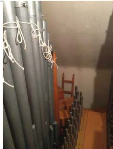
Figure 2: The walk board, and to the left are the small pipes of the Mixture II and the largest pipes of the 16' Trombone. A few of the horizontal 16' Contra Bass pipes can be seen at the back.
