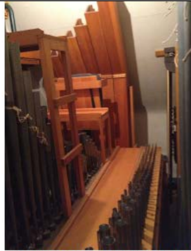
Figure 4: At the right is another view of the Mixture II. Against the back wall and angled are the largest pipes of the 8' Flute. They are mitered to follow the wall. Left of the walk board is the Trumpet.
